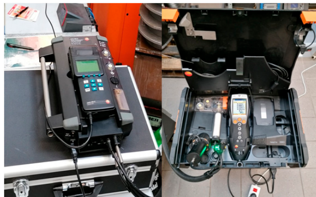
Figure 4. Exhaust gas analyzers used in tests. On left side: Testo 350s; on right side: Testo 380 and Testo 330-2 LL.
