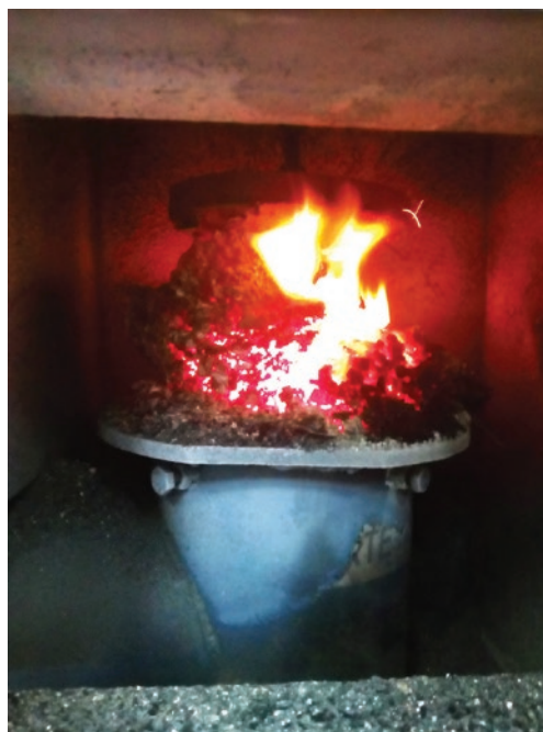
Rys. 3. Spiek żuźla w trakcie spalania węgla z owsem Fig. 3. Coke sintering during the combustion of coal with oats in a mixture
