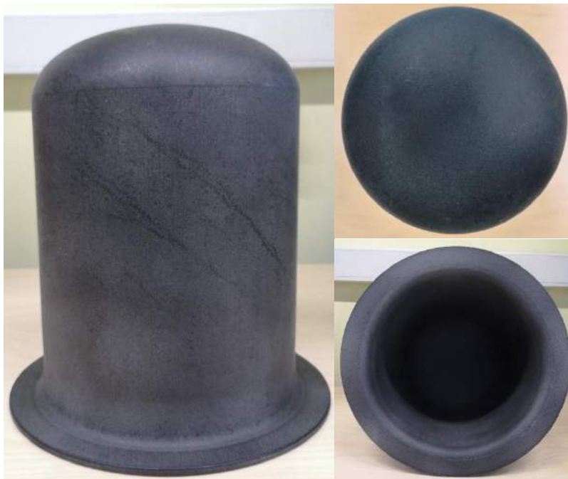
Fig. 7.23. The model of pressure vessel with optimized dished end manufactured in MJF technology
