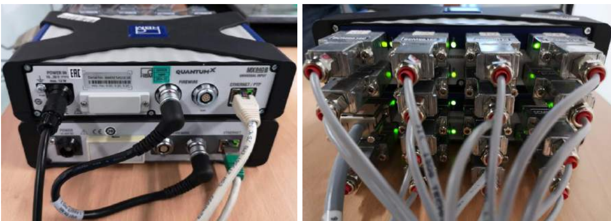
Fig. 7.13. Two HBM QuantumX MX840 amplifiers used for data acquisition
