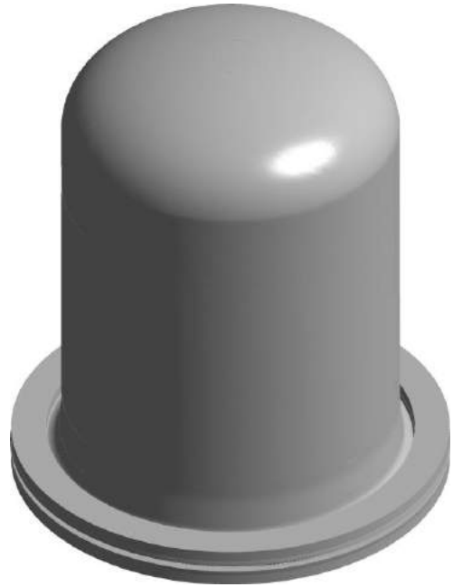
Fig. 7.42. The geometric model of the scanned pressure vessel
